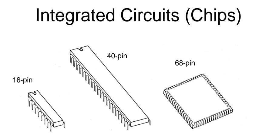
SSI: 1 to 10 gates LSI: 100 to 100,000 gates VLSI: more than 100,000 gates MSI: 10 to 100 gates
