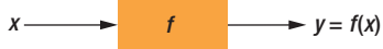
FIGURE 1. A functional perspective of a software system. The specification f defines how inputs ( x ) map to outputs ( y ). For distributed systems, such functional specifications are incomplete; they don't fully characterize a system's behavior for all possible inputs.
